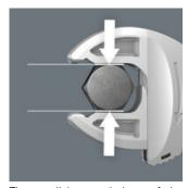
The parallel, smooth jaws of the 7880 Joker offer a seating stress and can thus prevent the nut or screw head from rounding, which can occur when power is transmitted over corners.
